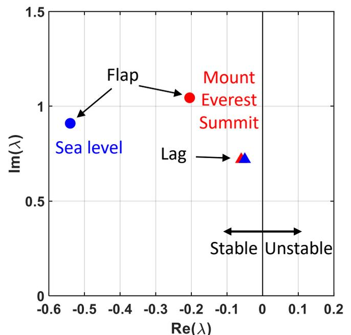
Elastomeric damper is selected for a possible **snow landing** which assures freedom from ground resonance for all terrain conditions.
