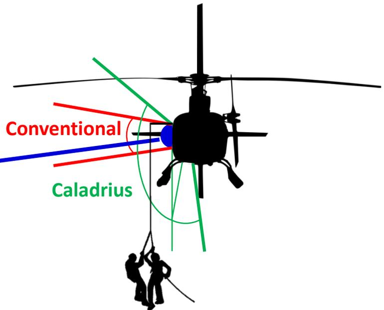
**Bubble window geometry was designed after extensive aerodynamic studies for minimal impact in aircraft drag and increased lateral field of view**
